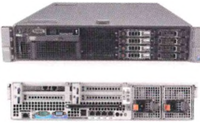
FIGURA 5 Server rack Dell PowerEdge R710
